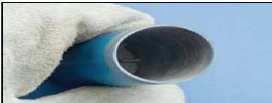
Fig. 21 The bottom of the tube contains compressed material (starting material). Tap the bottom of the tube a couple of times to loosen this material.
