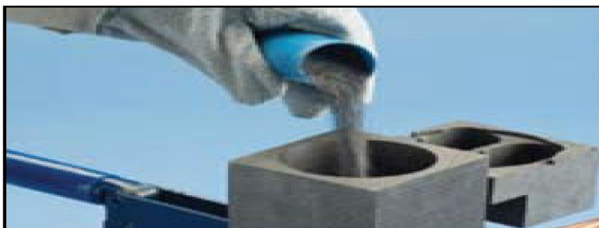
Fig. 20 Quickly pour the loose welding material powder into the mold.
